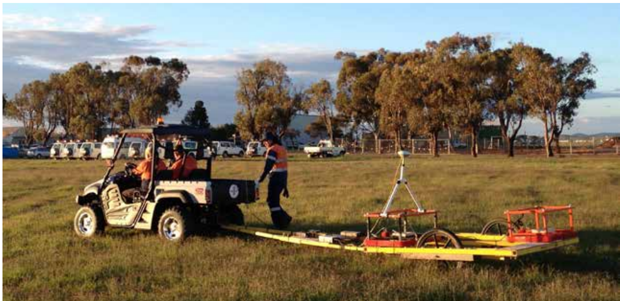
UXO detection using square loop Time-domain Electro-Magnetics TEM
