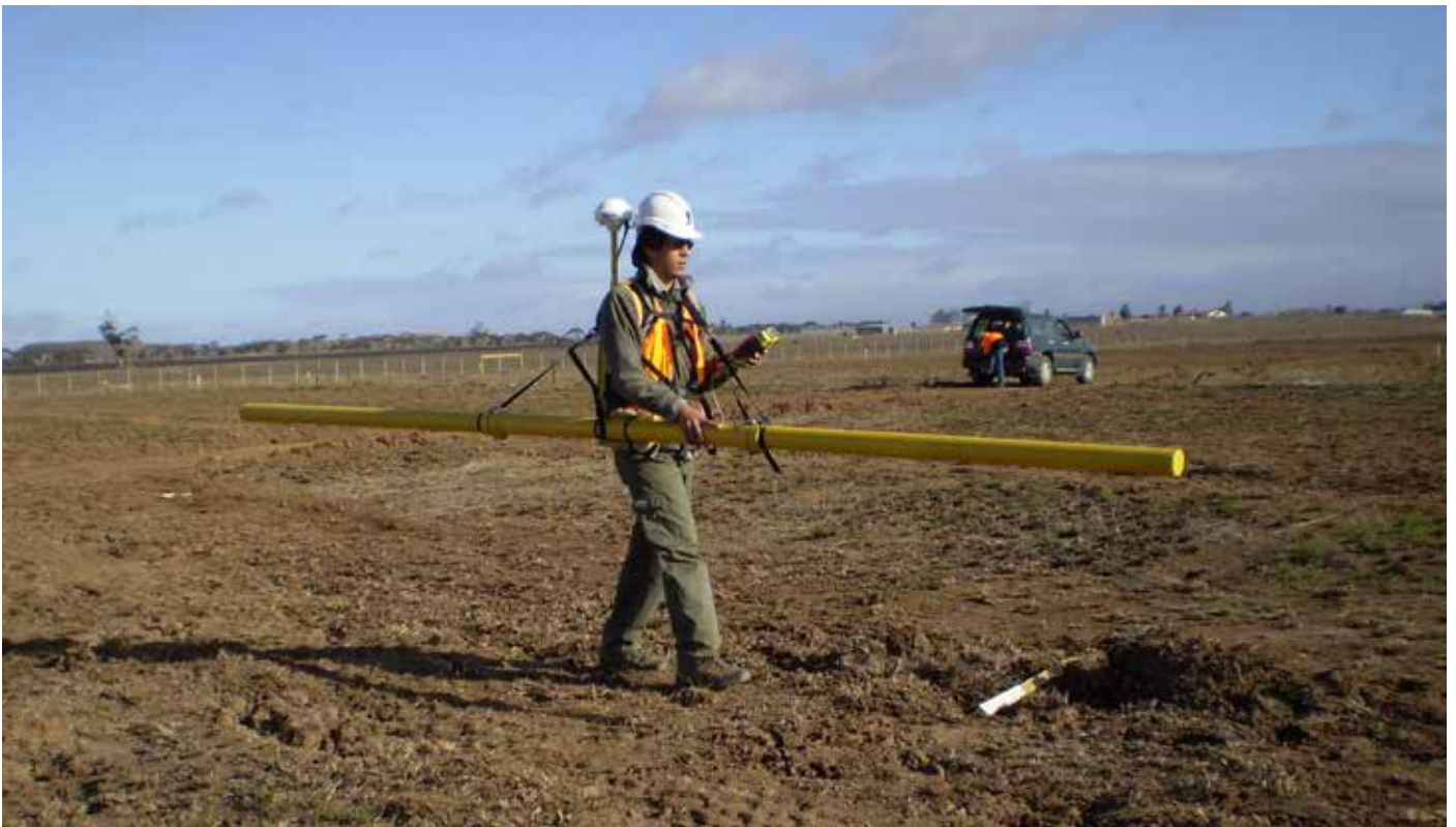
Mapping of soil contaminants at a former waste dump site using a Dual EM
